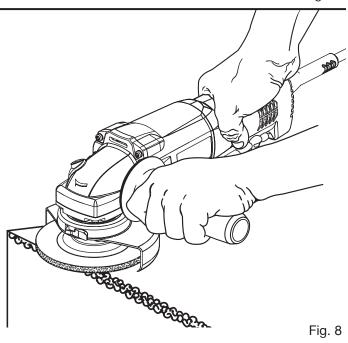
**NOTE:** Heavy pressure will decrease the grinder's speed and put a strain on the motor. Normally the weight of the tool alone is adequate for most grinding jobs. Use light pressure when grinding jagged edges or loose bolts where there is the potential for the grinder to snag on the metal edge.
